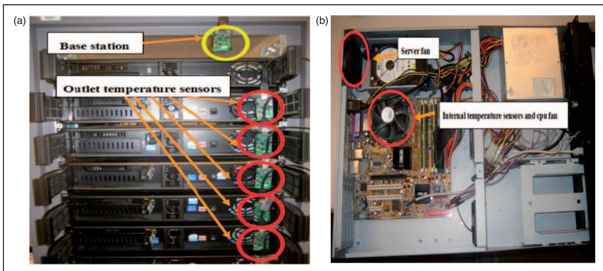
**Figure 5.** Location of sensors and fans: (a) wireless sensor network monitoring the outlet temperature of servers and (b) internal temperature sensors and fans around the heated elements on the motherboard.
