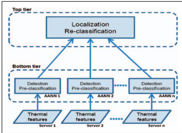
**Figure 1.** Information flow chart of our two-tier hierarchical NN framework. Thermal features are used to detect small-scale anomalies in the bottom tier, and the information is collected to detect large-scale anomalies in the top tier.
