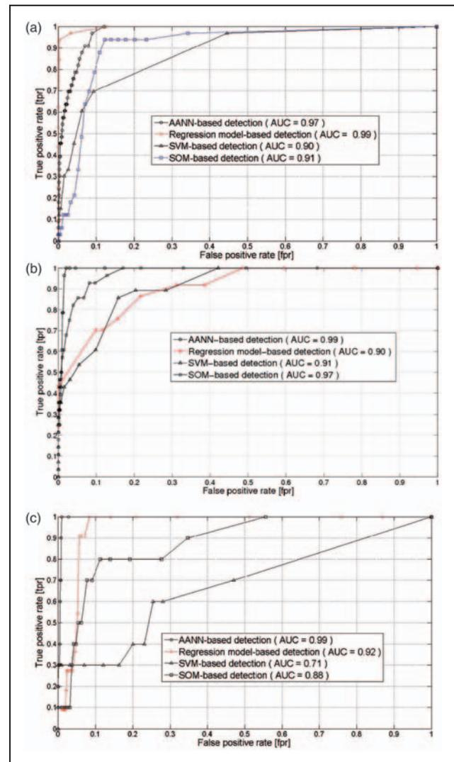
**Figure 8.** (a) ROC curve of the misconfiguration detection result with different approaches, (b) ROC curve of CRAC fan failure detection result with AANN using different approaches, and (c) ROC curve of server fan failure detection result with AANN using different approaches.
