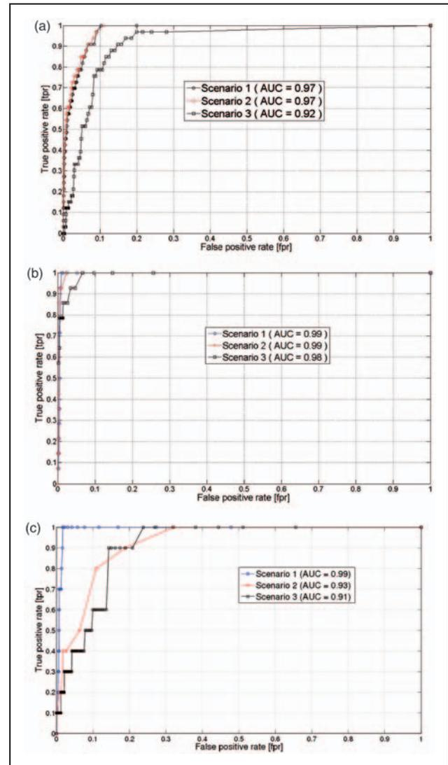
**Figure 7.** (a) ROC curve of the misconfiguration detection results with AANN using different features, (b) ROC curve of CRAC fan failure detection results with AANN using different features, and (c) ROC curve of server fan failure detection results with AANN using different features.
